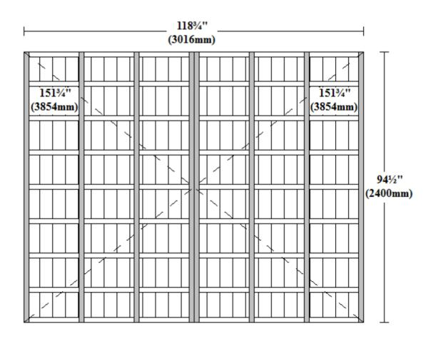
NB:- Floor joists run from left to right. Optional Floor Bearers run from front to back.
